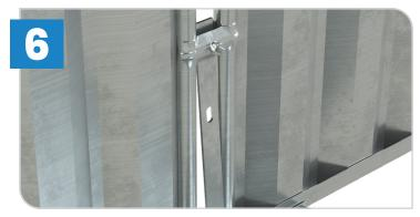
Use a coupler to secure the hinge at the front of the block tray to the two hoarding panels you're fixing together.
