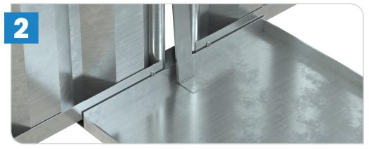
The block trays have a channel at the front. The steel panel is inserted into the channel. Don't secure the hinge in the block tray just yet, this can be done once the stabilizer arm is in place.
