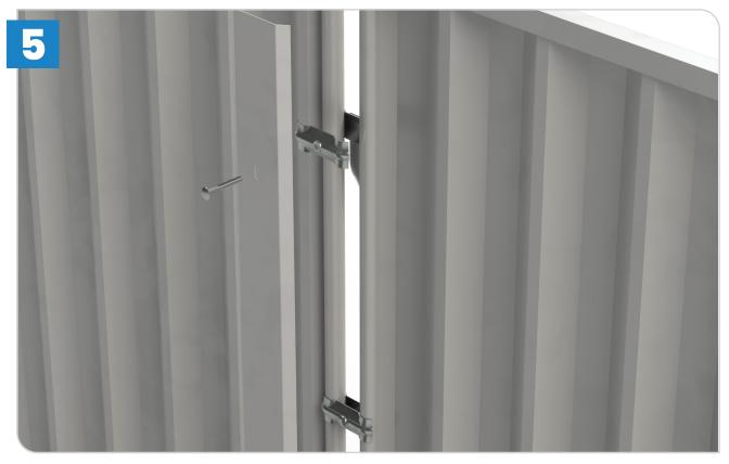
Next for 2m hoarding, install infill panels by filling the gaps between the hoarding. Simply thread the bolts of the top and bottom couplers through the holes on the infill panel. Tighten the couplers to affix it to the hoarding panels.
