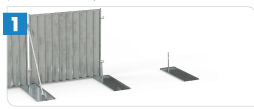
Lay the hoarding panels along the perimeter line.Position the block trays next to the edge of each steel panel, so that you have your panels and block trays in the right position, ready for the hoarding to be attached.
